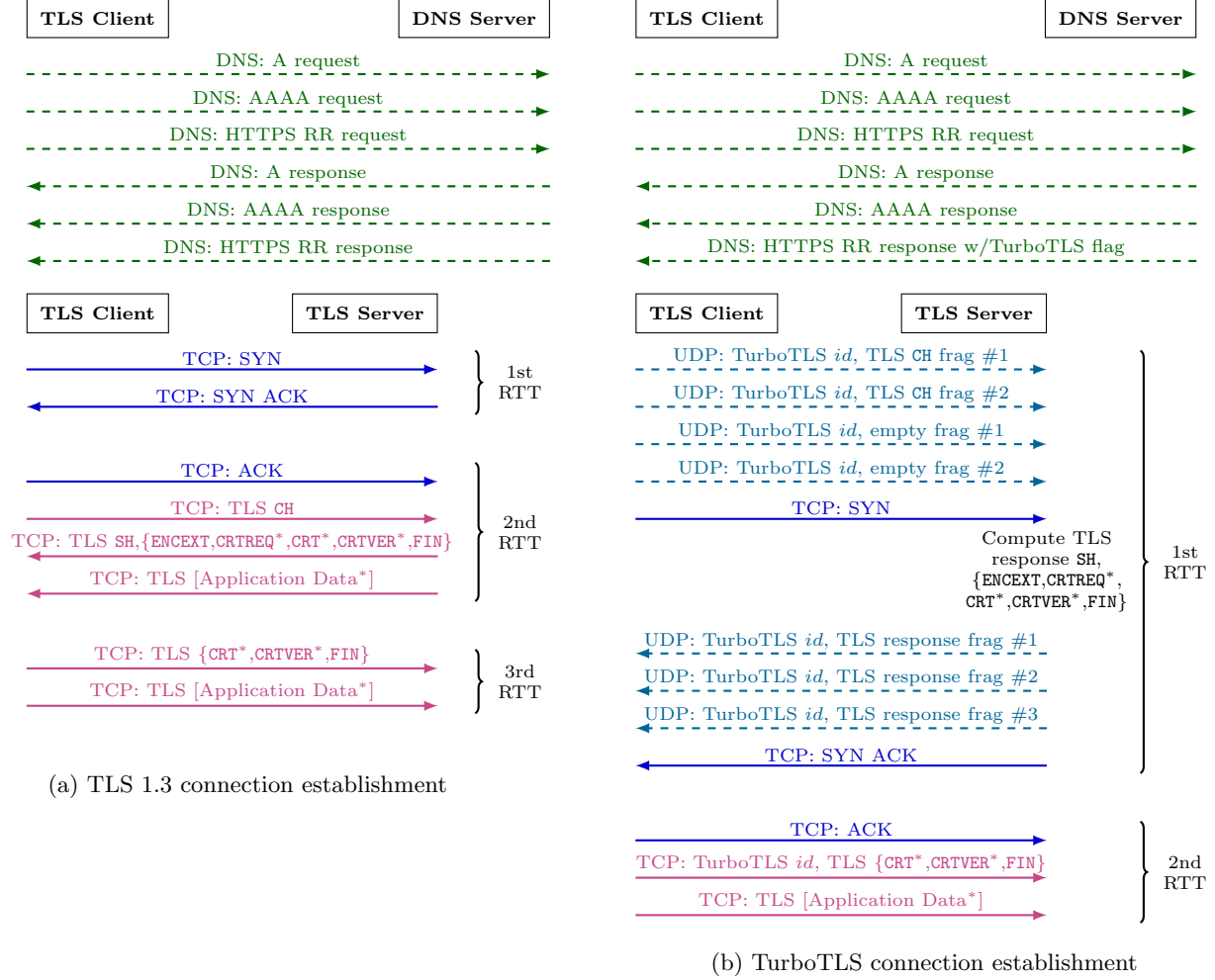
Figure 1: Comparing message flow of TLS 1.3 and TurboTLS. Legend: dashed line - UDP; solid line - TCP. * denotes optional message. {...} denotes messages encrypted using TLS handshake traffic secret and [...] denotes messages encrypted using TLS application traffic secret.
